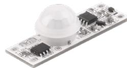
IN 12 Vdc - OUT 12Vdc 36W max
